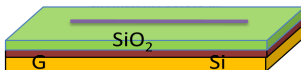
Figure 3: Single GaN-ZnO nanowire aligned between source and drain Ti/Au electrodes on \text{SiO}_2 /Si substrate.
